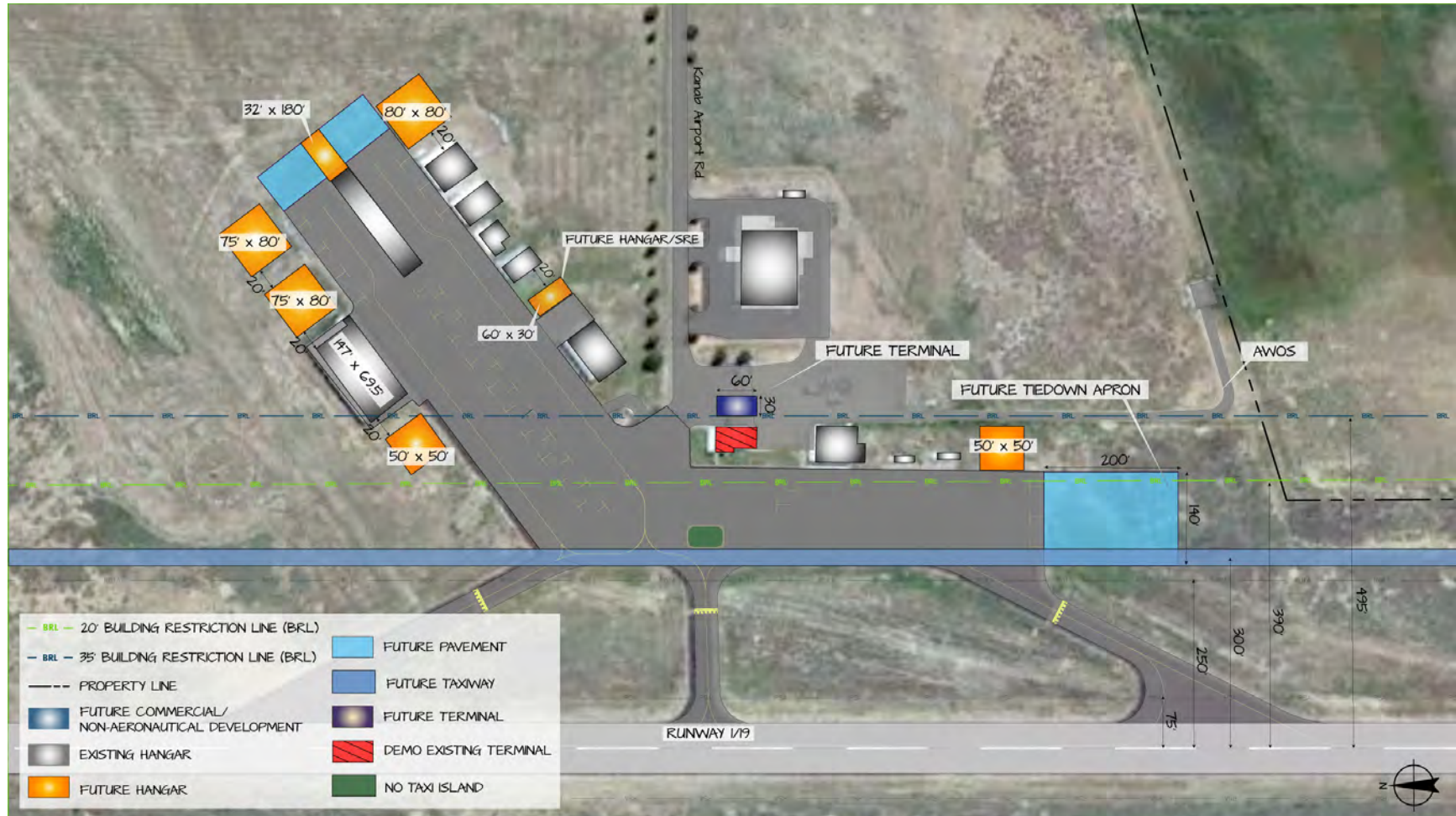
FIGURE 5-1 – KANAB MUNICIPAL AIRPORT – FUTURE TERMINAL LAYOUT
